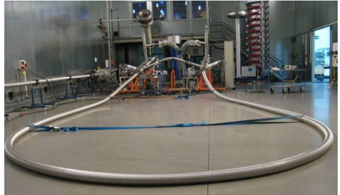
Cable superconductor 24kV-3200 A (Nexans-ICMAB). Barcelona (Premi Novare, 2012)
